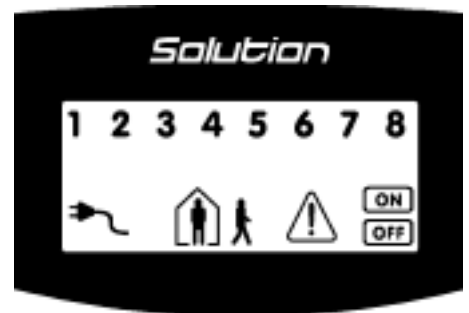
Figure 2: CP5 Eight Zone LCD Codepad
